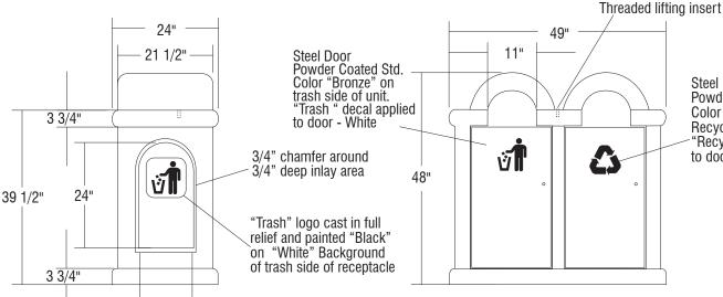
Steel Door Powder Coated Color "Recycle Blue" on Recycle side of unit. "Recycle" decal applied to door - White
