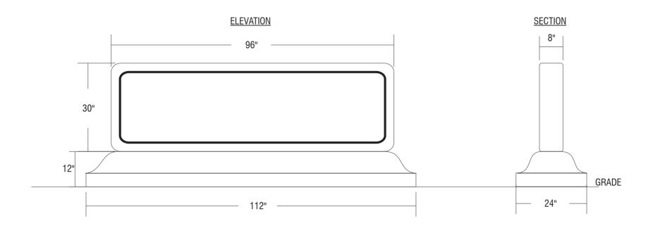
1. Concrete mix design to include a mixture of Portland Cement, water, coarse and fine aggregates, pure mineral oxide coloring agents (when applicable) to yield a minimum compressive strength of 5000 psi.
